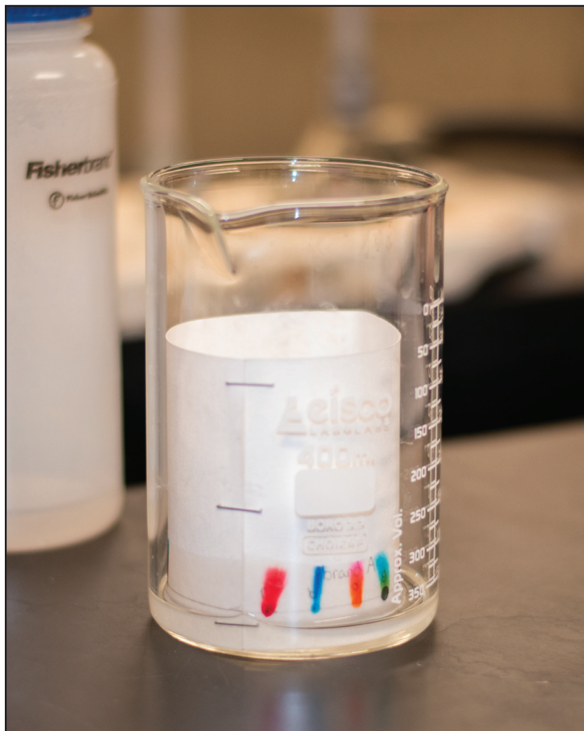
Color dots spread up a piece of paper based on their solubility in a mobile phase.
