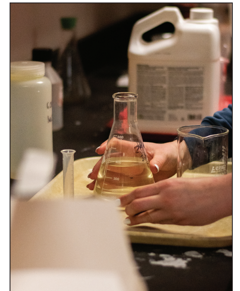
A student prepares a mobile phase of ammonia butanol and water.
