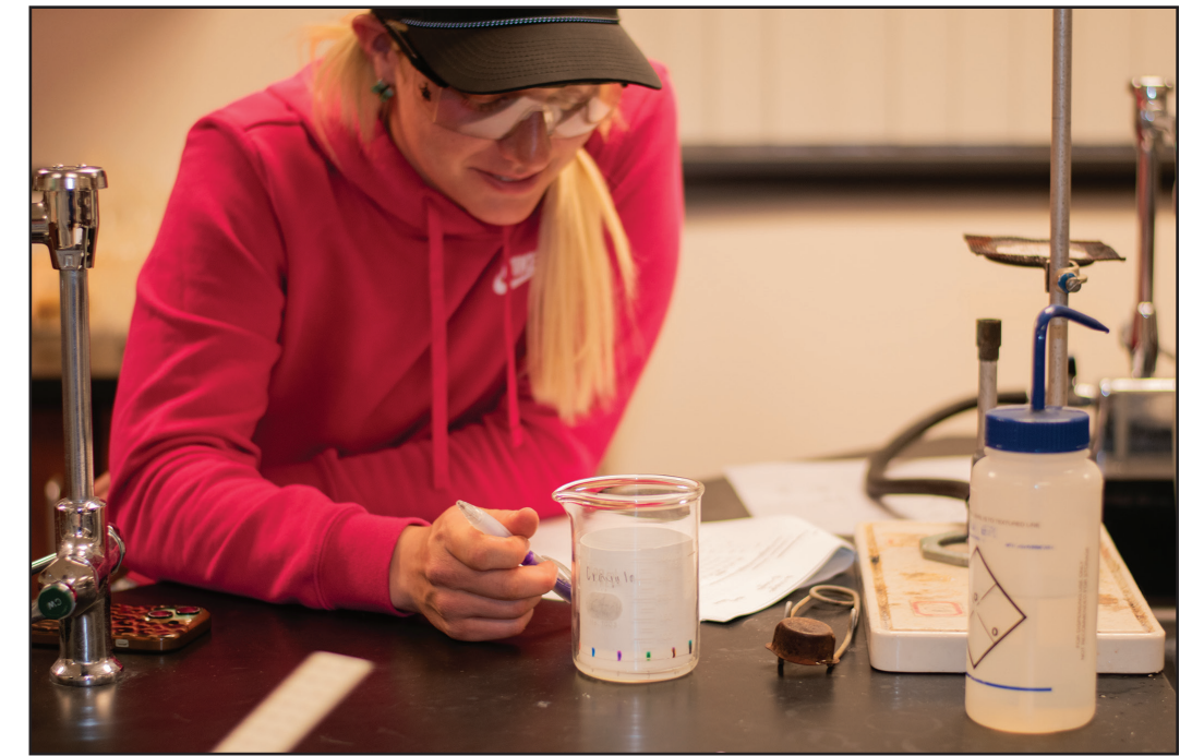
Savannah Greenfield placed color dots on a stationary phase into a beaker containing a mobile phase.
