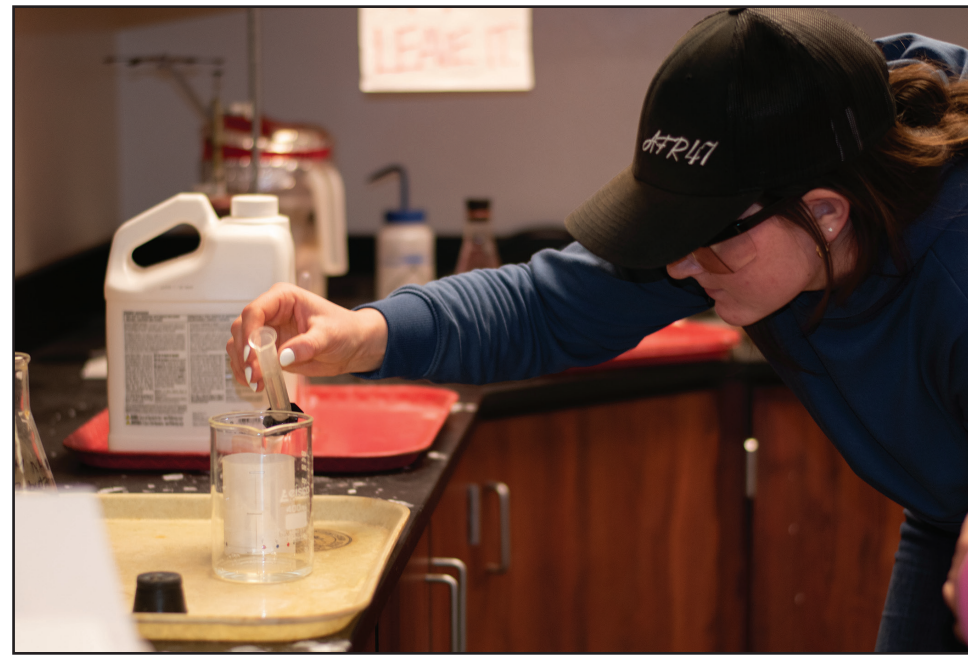
Emerson "Blue" Hall pours a mobile phase, made of ammonia, butanol and water, into a beaker.
